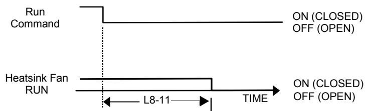
Fig. 97 Heatsink Cooling Fan Operation Timing Diagram
